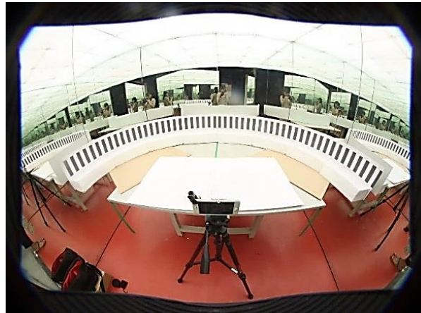
Figure 1 showing the experimental set-up for the vignetting correction of the fisheye lens used in the artificial sky simulator.
